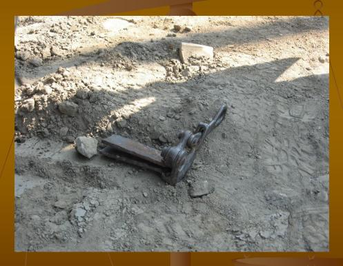
Wire rope clamp/puller modified to pull conveyor belting involved in a "near miss" incident.
