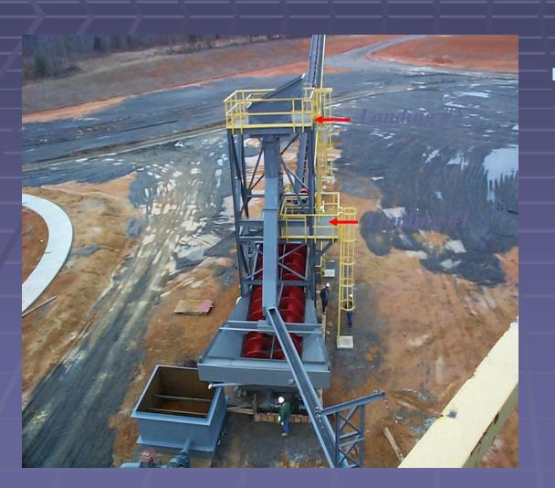
Fixed ladders must either be offset and constructed with a substantial railed landing at least every 30 feet, or, backguards must be provided.
