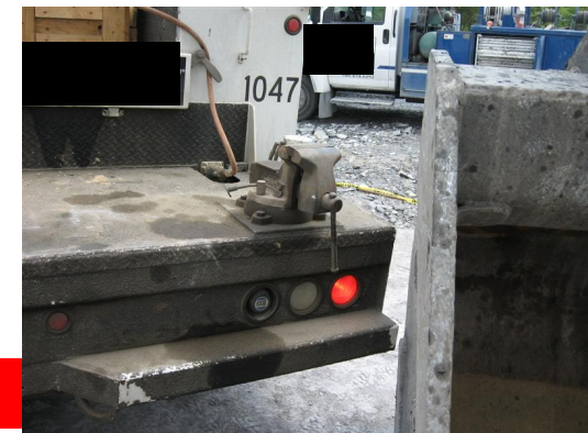
Pinch point between the bumper and bucket.
