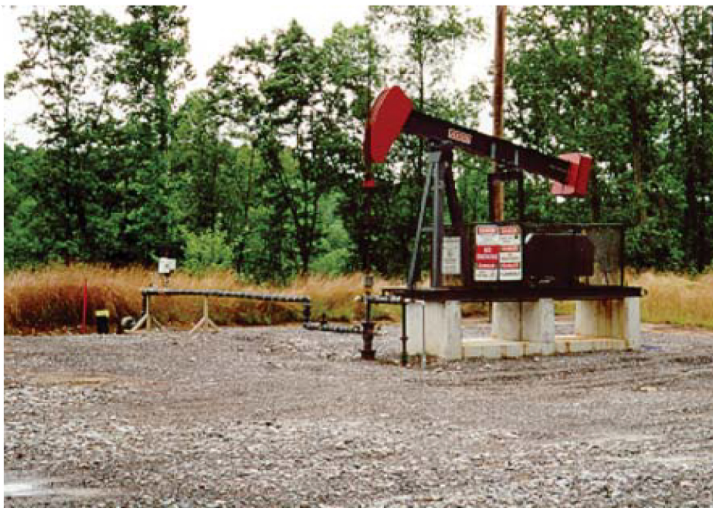
Pump jack installed on coalbed methane well operated by CNX Gas Company, LLC, in Buchanan County, VA. Photograph courtesy of the Division of Gas and Oil.
