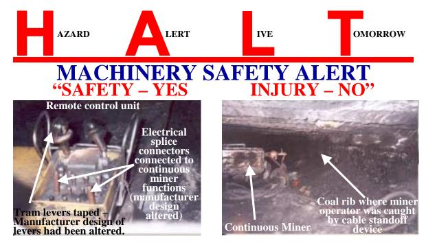
Machinery accidents continue to cause serious injuries and fatalities in the coal mining industry. Every person working in or around a coal mine must always stay alert to potential accident hazards when working around machinery. A continuous miner operator with only limited remote control miner operation experience at this mine received fatal injuries when he was pinned between the continuous miner cable standoff device and the coal rib. (photo's above)
