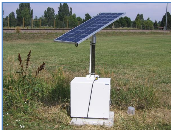
Figure 6-1 A solar-powered Air Sampling System
