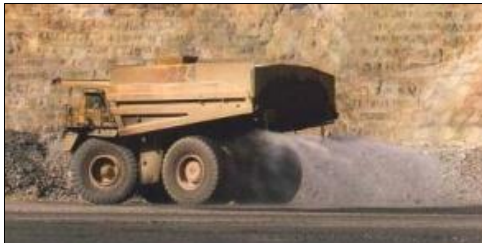
Figure 4-3 Example of Dust Control Using a Water Truck
