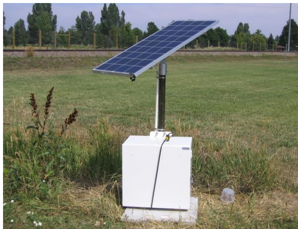
Figure 2-1 A Current Solar-Powered Air Sampler System (Sampler filter head is mounted directly under the solar panel)
