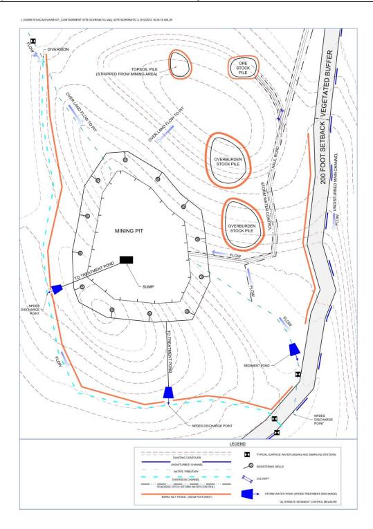
Figure 2-1 Conceptual Storm Water Runoff Site Schematic
